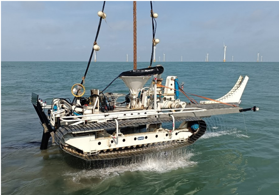
Figure 3.13 Shallow water trencher (source: https://www.smd.co.uk/blog/may-2023-smds-shallow-water-trencher-the-story-so-far/ )
