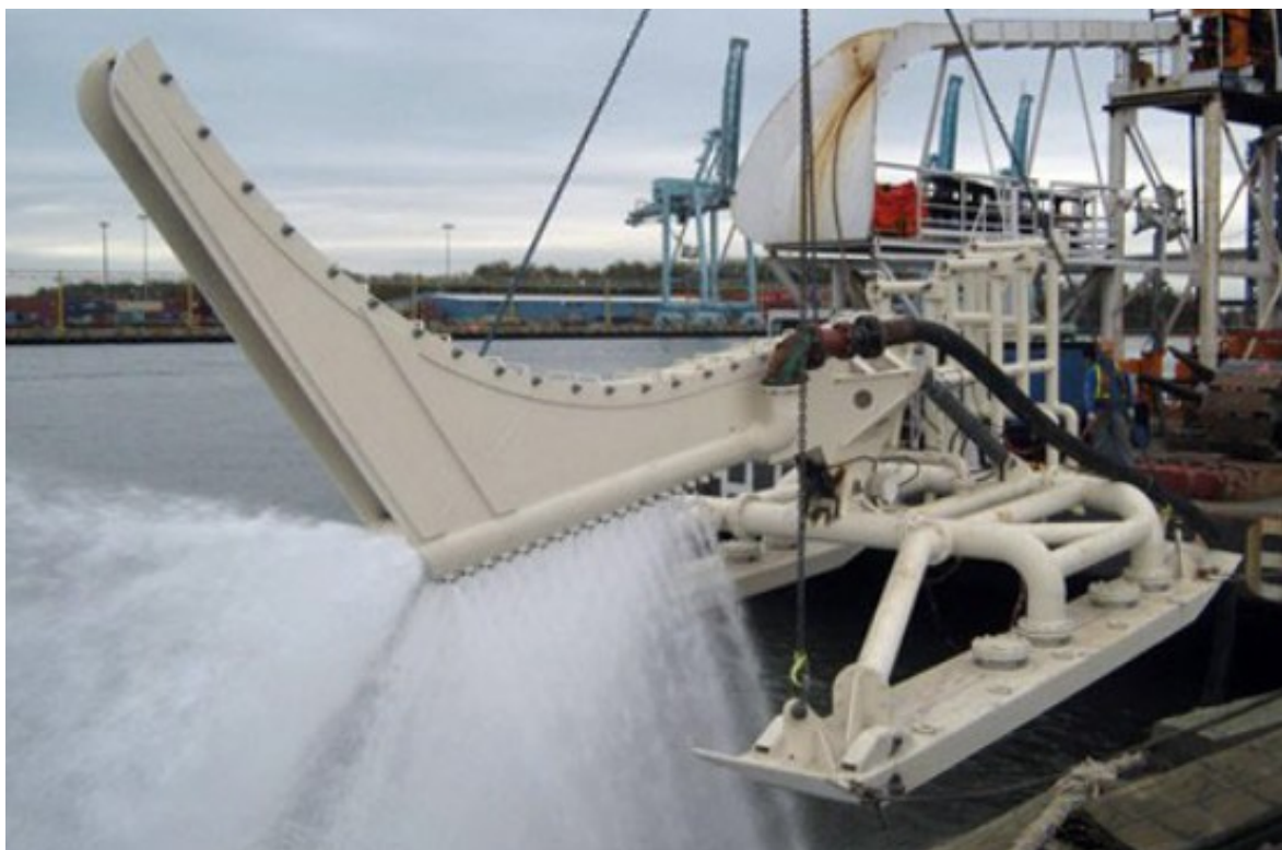
Figure 3.12 Sleds for power cable laying for the Mod-Jet/Sea Venture (source: https://eta-ltd.com/jetting-sleds-for-subsea-power-cable-laying/ )
