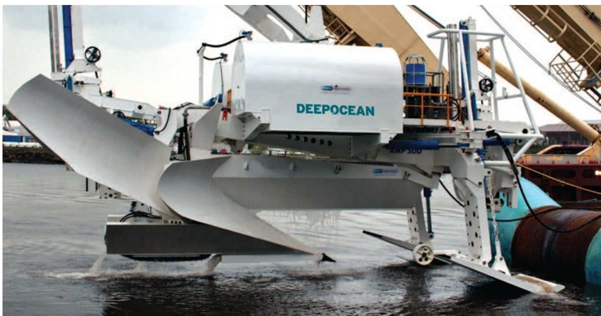
Figure 3.15 AMP500 advanced multi-pass plough. Source: https://www.subsea-rov.com/services-assets/trenchers-ploughs/item/74-amp500
